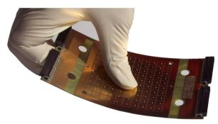
The sensor plate shown above has a thickness of 0.7mm.
