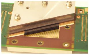
If necessary the gas diffusion layer can be placed directly on the segments. Therefore the channels of the flow field can be milled between the segments. The device is usable as anode or cathode of a single cell.
